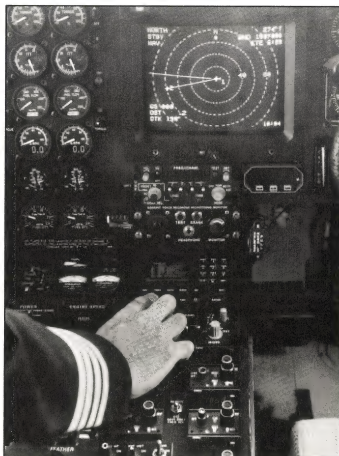
Racal Avionics RNS 5000 worldwide navigation management system – Above left: Installed in an Embraer Brasilia aircraft. Above right: Installed in a major civil aircraft.
